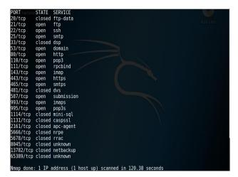
Figure 4. Nmap result after scanning
